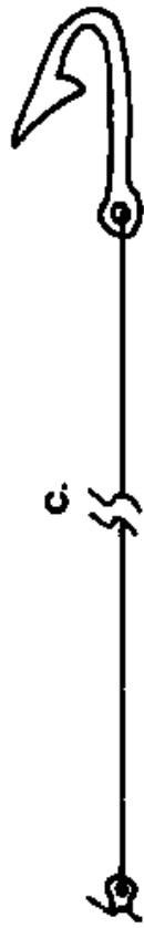
ATTACH KUSARI-GAMA BLADE WITH TWO 1/4" x 1 1/2" WOODEN DOWELS & CLAMPS
